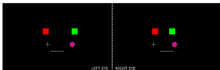
Figure 9: Fake 3D example. The left half of the image is sent to the left eye, and the right half to the right eye.
