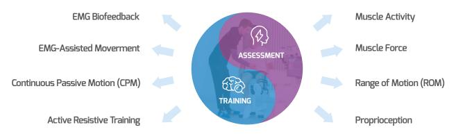
The most unique feature - **EMG-assisted movement.\*** - active training, even for very weak patients (MMT 1) \*EMG = electromyography, electrical activity of the muscle. Robot detects the patient's muscle activity via sensors and converts it into intended movement.
